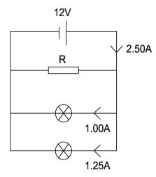
Calculate the power dissipated by resistor R.
