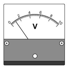
Name the type of error on the voltmeter and suggest how it should be dealt with.
